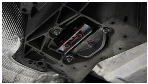
**Step 3**Remove the factory transmission mount bracket.
