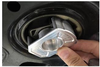
Step 4 Using the 21mm socket, install a **new** factory bolt. Torque to 130Nm+90°.
