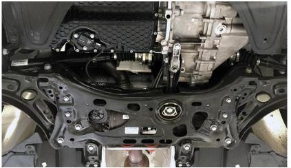
**Step 2** Using the 21mm socket, remove the factory bolt.
