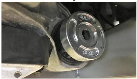
**Step 12**Reinstall the through bolt on the rear bushing brace.
