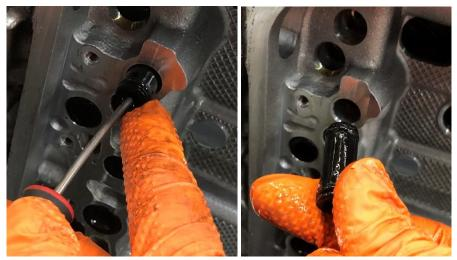
**Step 10**Apply a small amount of oil to the 034 oil tubes.
