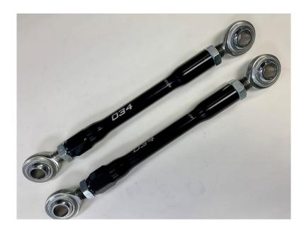
You are now ready to start the installation process. Use the length of the stock component as a starting point for the length of the 034 adjustable end links; expand or compress as best fits your needs
