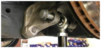
**Note**: Use the short spacers are on the hub assembly and the taller spacers on the rear subframe. To make adjusting easier, the hex end of the tube should connect to the subframe.
