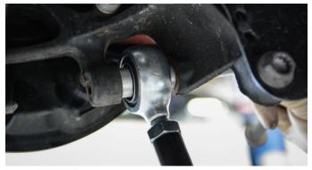
\*Position such that the short spacers are on the outside (hub assembly) and taller spacers mount to the rear subframe
