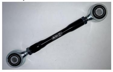
**Step F**Install (2x) spacers into each Density bushing.
