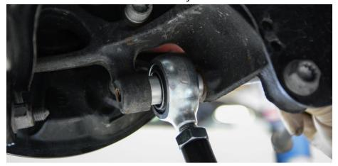
\*Position such that the short spacers are on the outside (hub assembly) and taller spacers mount to the rear subframe.
