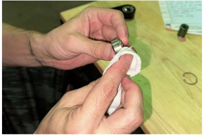
**Step 5** Push the bearing into the bore, checking your alignment.
