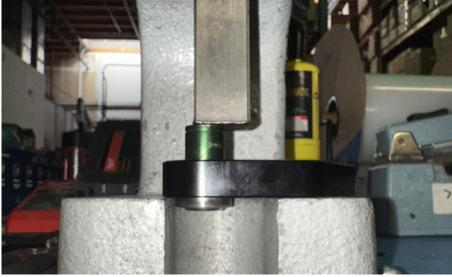
**Step 3** Thoroughly clean the bore where the old bearing was secured.
