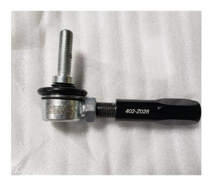
You are now ready to start the installation process. Use the length of the stock component as a starting point for the length of the 034 adjustable end links; expand or compress as best fits your needs
