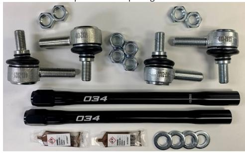
**Step B**Apply half packet of anti-seize to each spherical heim joint
