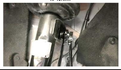
**Note**: the orientation of the link is such that the 19mm hex on the connecting rod is pointing downward during installation.
