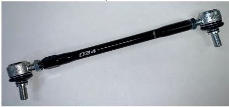
Use the length of the stock component as a starting point for the length of the 034 adjustable end links; expand or compress as best fits your needs
