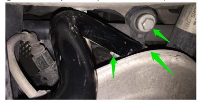
\*We recommend replacing the factory end link bolts as they are torque-to-yield bolts.
