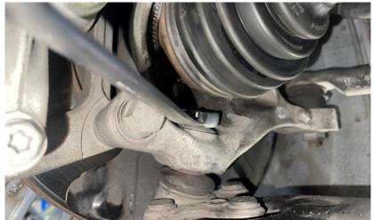
\*To prevent the ball joint stud from spinning, use a 7mm Allen on the top of the stud. This will require moving the axle out of the way. Alternatively, you can loosen the nut with the wheels still on, and under load.
