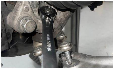
\*If you moved the axle out of the way, a T40 Torx will fit into the end of the stud to keep it from spinning.
