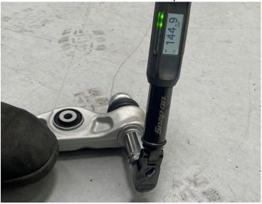
**Step 19** Install the 034 "front" lower control arm assembly into the upright.
