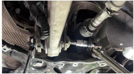
**Step 16** If the steering rack is still obstructing the bolt from being removed, use a pole jack to lift the hub assembly.
