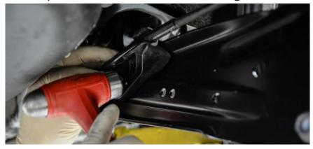
**Step 22**With a hammer and punch, tap the securing pin into metal retainer.
