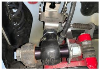
**Step 10**Attach the ABS sensor wire to the bracket on the 034 arm.
