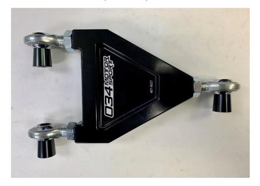
Use the length of the stock component as a starting point for the length of the 034 adjustable rear upper control arms; expand or compress as best fits your needs
