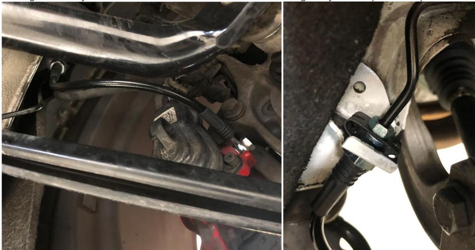
Finish up by bleeding the brakes. This will take 1-2 quarts depending on how much brake fluid was lost when installing the brake lines. Inspect the lines for leaks as you bleed the brakes.
