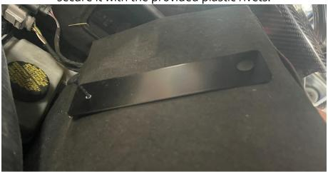
**Step 15**Trim the excess tails from the plastic rivets.
