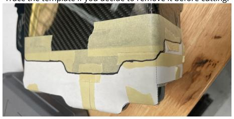
**Step 7**Using a rotary cutting wheel, carefully start trimming.
