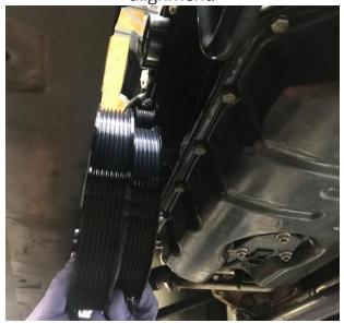
Install the M8x25 socket head cap screws finger tight. Once all are installed, torque to **30Nm** (22 ft-lbs).
