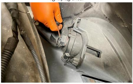
**Step 54**Reinstall the crash sensor plug.
