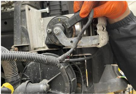
**Step 27**Remove the impact sensor from the crash bar.
