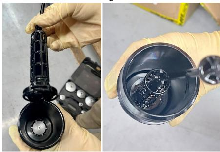
**Step 7**Slide the oil filter over the filter support tube.
