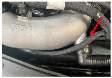
**Step 16** Attaching the vacuum line fitting to the turbo inlet is a bit tricky, take your time and push the fitting onto the turbo inlet. (Fitting is under the inlet)
