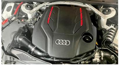
**Step 2** Remove the engine cover by pulling up on it.
