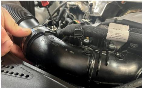
**Step 4** Slide the hose off of the turbo inlet.
