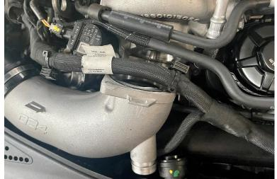
**Step 14** Using a 5mm Allen, tighten both bolts to secure the 034 turbo inlet to the turbo.
