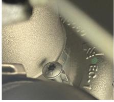
**Step 27**Reinstall the wastegate hardline to the wastegate.
