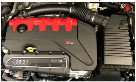
**Step 2**Remove the engine cover.
