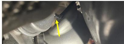
**Step 19**Disconnect the wastegate hardline near the coils and set aside.
