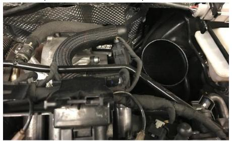
**Step 11**Install the Performance Drop-In Air Filter.
