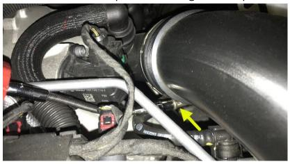
**Step 4**The stock inlet hose can now be pulled out.
