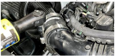
\*This next bit takes some finesse as the air filter/tube will want to disengage from the airbox grommets while moving around. Use soap to keep the grommets in place when installing the appropriate carbon components.
