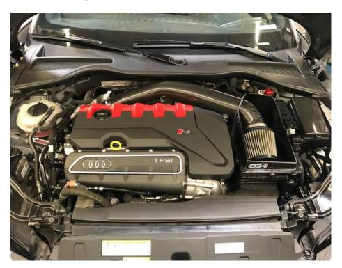
**Step 2**Remove the engine cover by pulling upward.
