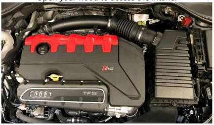
**Step 2**Remove the engine cover by pulling it up.
