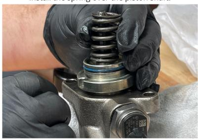
**Step 27**Reinstall the spring retainer
