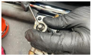
**Step 15**Remove the fuel pump spring.
