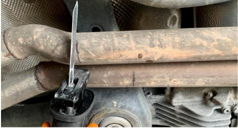
**Step 5** Remove the freshly cut factory exhaust by loosening the (4x) 13mm bolts at the exhaust junction.
