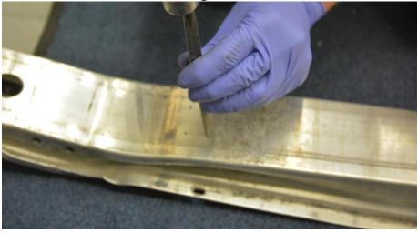
Using an <sup>1</sup>⁄<sub>8</sub>" drill bit, drill out the holes.
