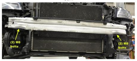
\*You may have to pry between the bumper bar and frame rails to loosen enough to slide out.
