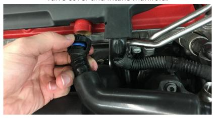
**Step 4**Insert the plug into the hole.
