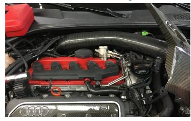
**Step 2**Locate the breather hose between the valve cover and intake manifold.
