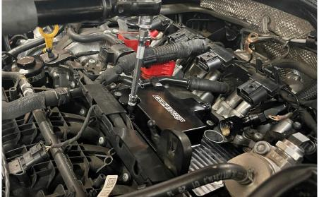
**Step 25** Using a 16mm Socket, remove the bolt securing the front of the motor mount to the chassis.
