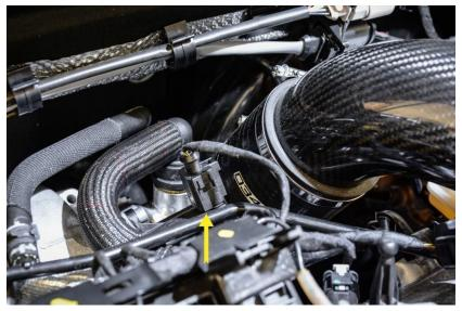
**Step 9** Disconnect the High Pressure Fuel Pump (HPFP) connector.
