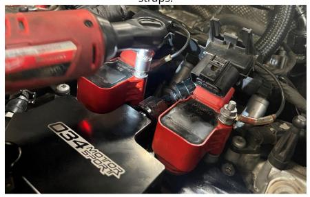
**Step 43** Reinstall the coil connectors.
