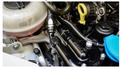
**Step 37** Connect the AN line to the 034 breather plate and tighten it with a crescent wrench.
