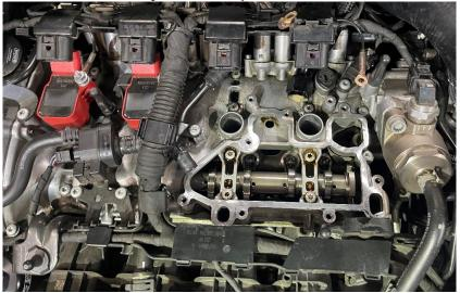
**Step 18** Transfer the sealing gasket over to the 034 breather plate.
