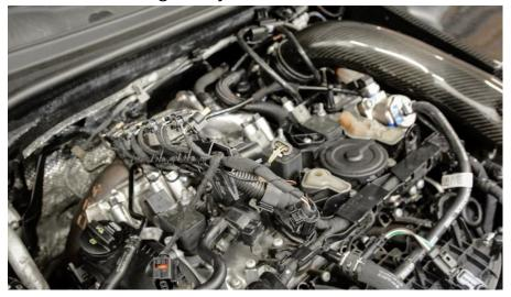
**Step 13** Using a 10mm Socket, remove the stud securing the two coils furthest to the right and remove.
