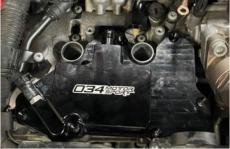
**Step 23** Using a 4mm Allen, secure the 034 breather plate to the valve cover.
