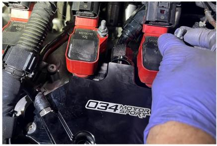
**Step 41** Reinstall the ground straps onto the studs.
