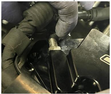
**Step 22** Place the 034 breather plate into the factory location.
