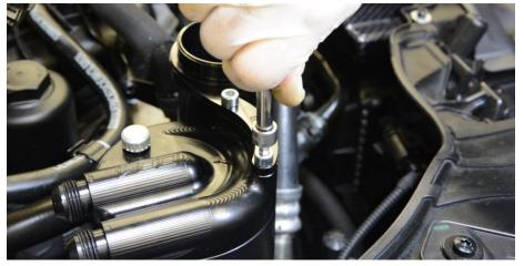
**Step 33** Transfer over factory washer fluid screen and cap to the newly installed filler neck.
