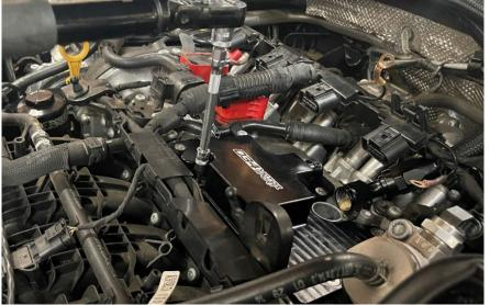
**Step 25** Using a 16mm Socket, remove the bolt securing the front of the motor mount to the chassis.
