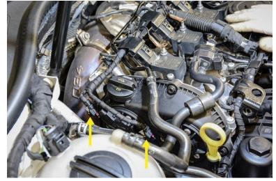
**Step 7** Disconnect the Valve Solenoid Connectors. There should be 8 in total.
