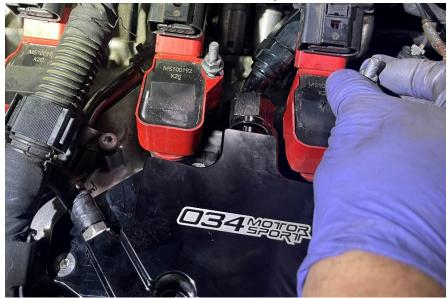
**Step 35** Reinstall the ground straps onto the studs.
