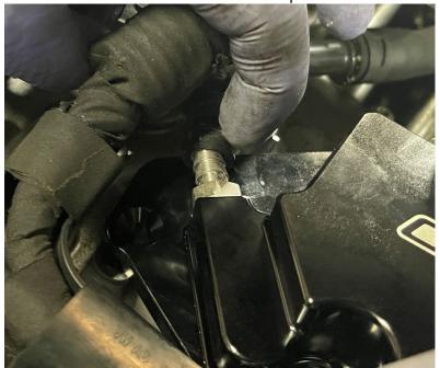
**Step 22** Place the 034 breather plate into the factory location.
