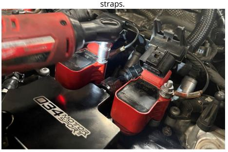
**Step 37** Reinstall the coil connectors.
