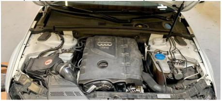
**Step 2**Remove engine cover by gently pulling upward.
