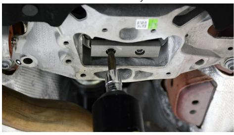
**Step 3**Remove the factory transmission mount bracket.
