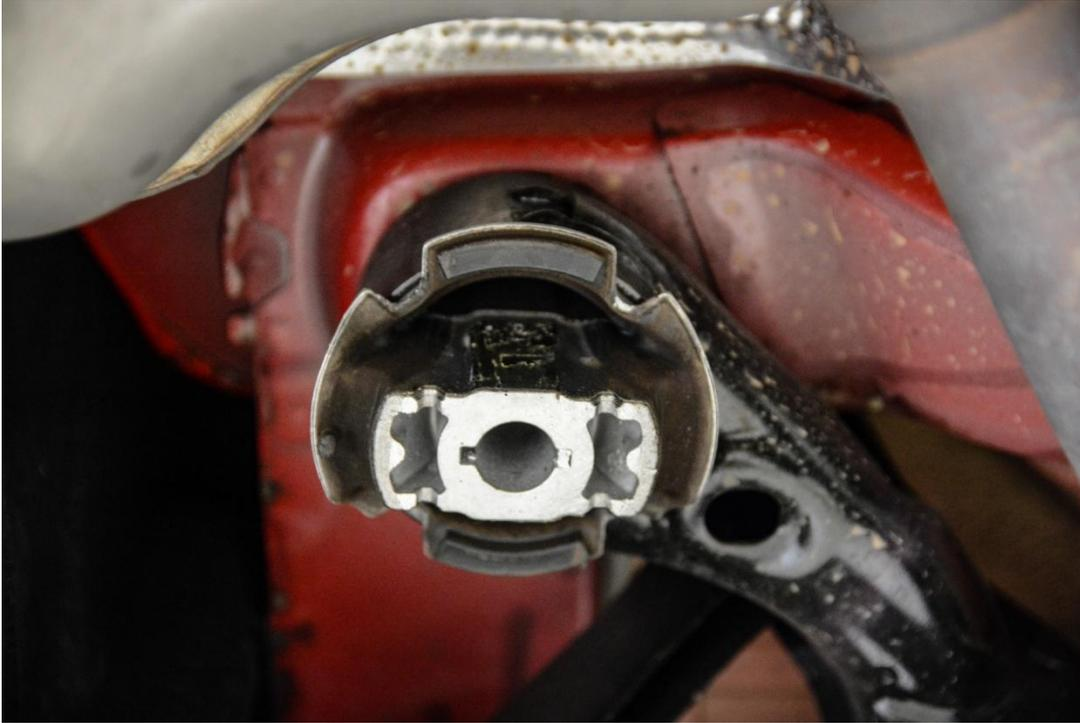
**Step 16** - Apply a coat of grease to the Rear 034Motorsport Billet Aluminum Rear Subframe Insert. (PN: 601-0045)
