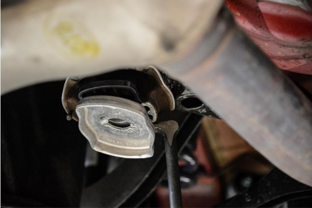
**Step 14** – Remove the black plastic collar from the rubber bushing.
