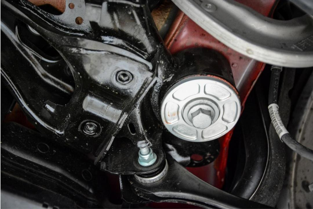
**Step 12** – Using an 18mm socket, loosen and remove the factory bolt securing the rear bushing of the rear subframe to the chassis.
