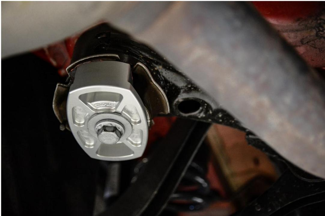
**Step 19** - Once all four 034Motorsport Billet Aluminum Rear Subframe Inserts are installed and torqued to spec, reinstall the rear sway bar, beginning with the mounting brackets. **Note:** Hardware may differ from factory rear sway bar for aftermarket bars.
