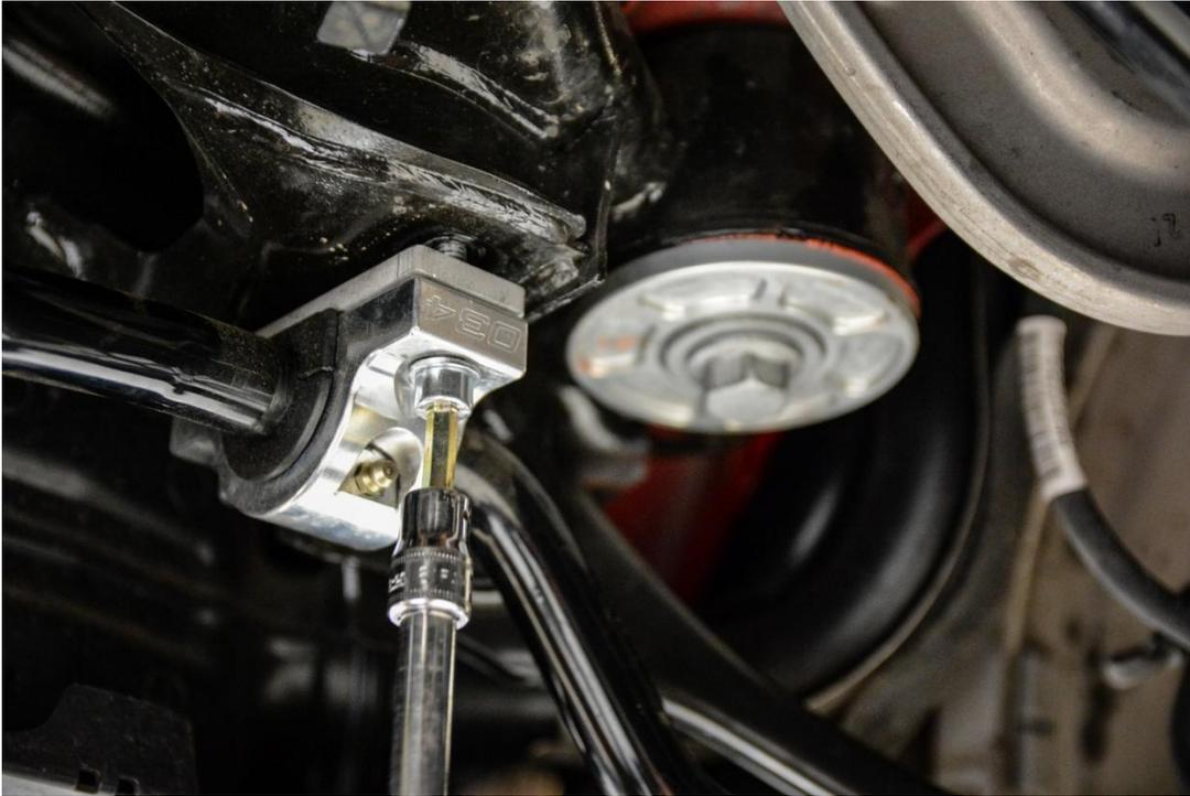
**Step 20** - Reattach rear sway bar to rear sway bar end links. Torque end link hardware to **40Nm + 180 Degree Turn**. Torque rear sway bar mounting bracket bolts to **28 Nm**.
