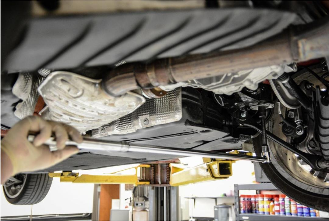
**Step 6** – Once the bolt is removed, use a pry bar to remove the factory metal collar from the rubber bushing.
