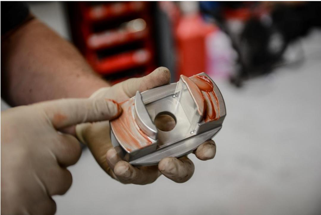
**Step 17** - Insert the Rear 034Motorsport Billet Aluminum Rear Subframe Bushing Insert into the factory rubber bushing, and secure using the factory subframe bolt and an 18mm socket. Torque to **90NM + 180 Degree Turn**.
