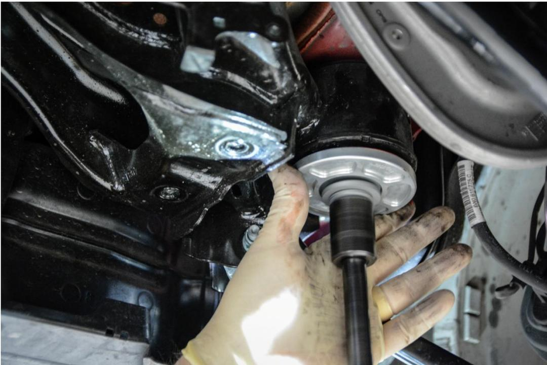
**Step 11** – Torque to **130 NM + 180 Degree Turn.**
