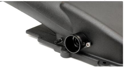
For Golf R and S3 owners, install the provided block-off plate on the side of the air box using the supplied Allen bolt.
