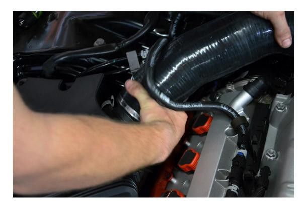
**Step 9** – Attach the small vacuum hose from Step 5 onto the new 90 degree nipple in the 034Motorsport Silicone Throttle Body Inlet Hose.
