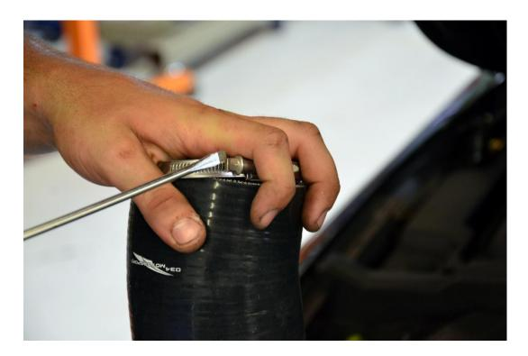
**Step 8** – Install the 034Motorsport Silicone Throttle Body Inlet Hose onto the throttle body and airbox.
