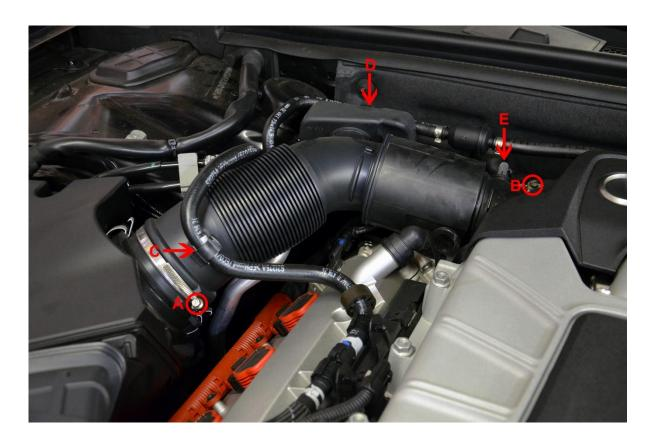
**Step 3** – Use flathead screwdriver or hose clamp driver to loosen the hose clamps, labeled A and B.
