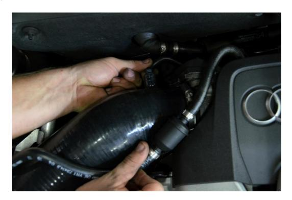
**Step 10** – Tighten both hose clamps at the throttle body and airbox.
