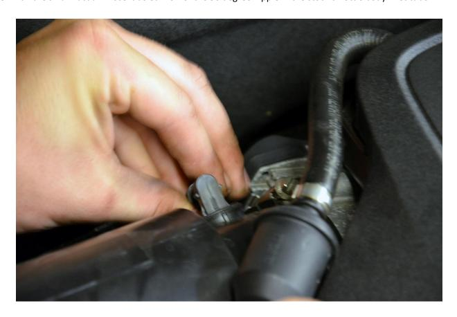
**Step 6** – Remove the stock throttle body inlet tube from the throttle body and airbox, and set aside.
