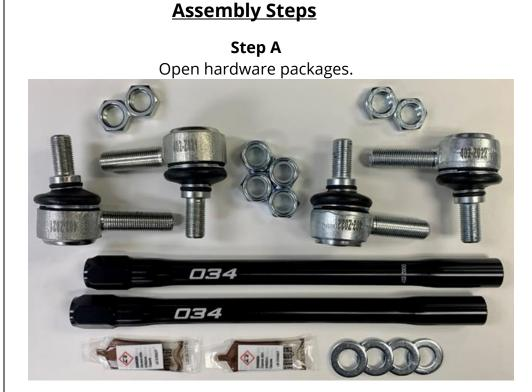
**Step B** Apply half packet of anti-seize to each spherical heim joint
