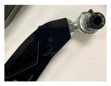
\*Please note that the 401-Z016 spacer is associated with the spherical heim joint, and the 401-Z015 spacer is associated with the spherical bearing
