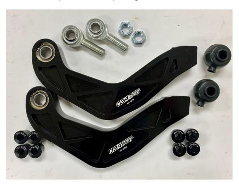
Apply half packet of anti-seize to each spherical heim joint
