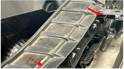
**Step 18** Attach the fuel line clip back to the valve cover.
