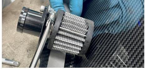
**Step 4** Insert the intake hose into the heat shield. Attach appropriate hose clamps on both ends.
