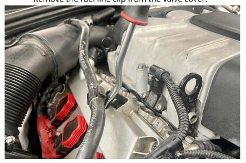
**Step 6** Unclip the fuel lines from the intake hose.
