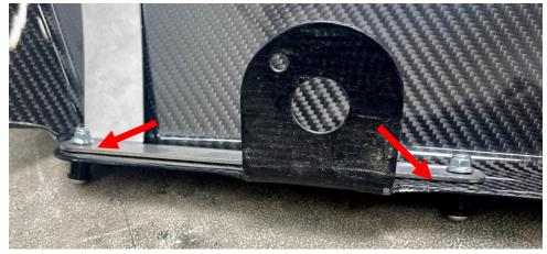
**Step 2** Using a 4mm Allen and an 8mm socket, attach the SAI adapter to the heat shield.
