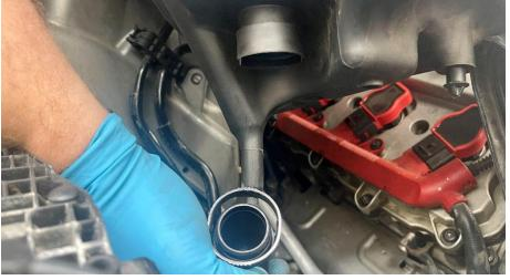
**Step 12** Remove the airbox from the vehicle.
