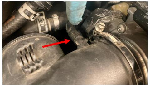
**Step 8** Using a flathead screwdriver, loosen the hose clamp near the throttle body.
