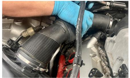
**Step 10** Separate the intake air duct from the airbox.
