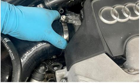
**Step 16** Attach the SAI fitting to the adapter.
