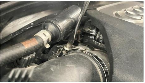
**Step 9** Separate the intake hose from the throttle body.
